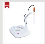
> Misuratore da banco pH, ORP, Ioni, Temperatura calibrazione 1-5 punti (pH range -2.00 - 20.000 pH, accur. +/-0.002pH, ris. sel. 0.1-0.01-0.001pH) (mV range 1999.9-1999.9mV, accur. +/-0.2mV, ris. sel. 0.1-1mV) (Ion conc. range 0.001-19999ppm, mg/L, mol/L, accur. +/-0.5% F.S monovalente +/-1% F.S bivalente) (Temp. range 0-105°C, 32-221°F, accur. +/-0.5°C +/-0.9°F) Conserva fino a 500 dati, Connessione USB, Display LCD
